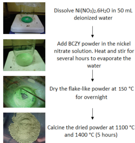
FIGURE 1. Steps for the preparation of NiO-BCZY composite powder by EDSS method
