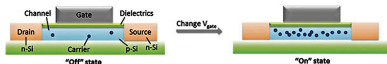
FIGURE 12. A typical planar field effect transistor (Zhang & Zheng 2015)
